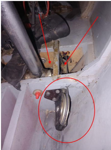
Fig. 9 – Rudder pedal control pulley on bulkhead No. 2
