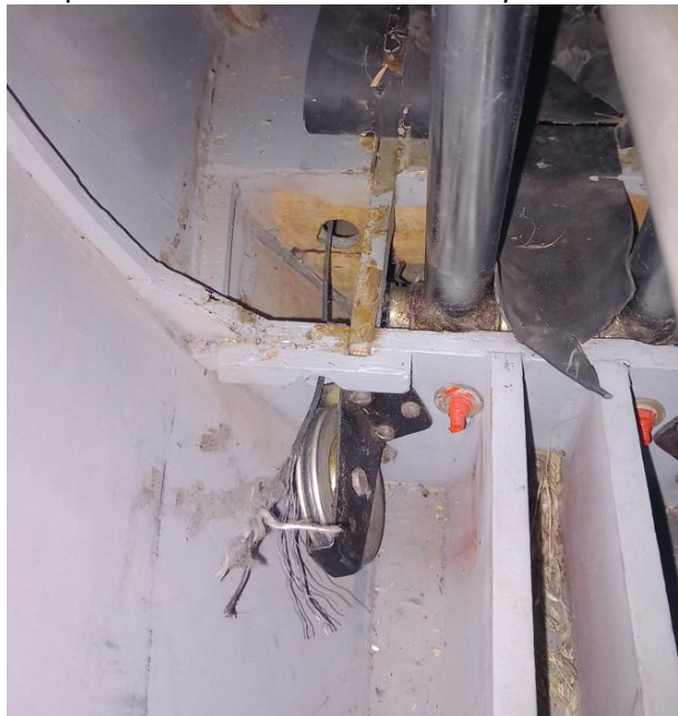
Fig.1 – Fractured rudder control cable
