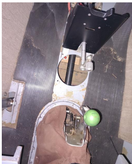
Fig. 5 – Circular cover in the cockpit floor between bulkheads Nos. 3 and 4
