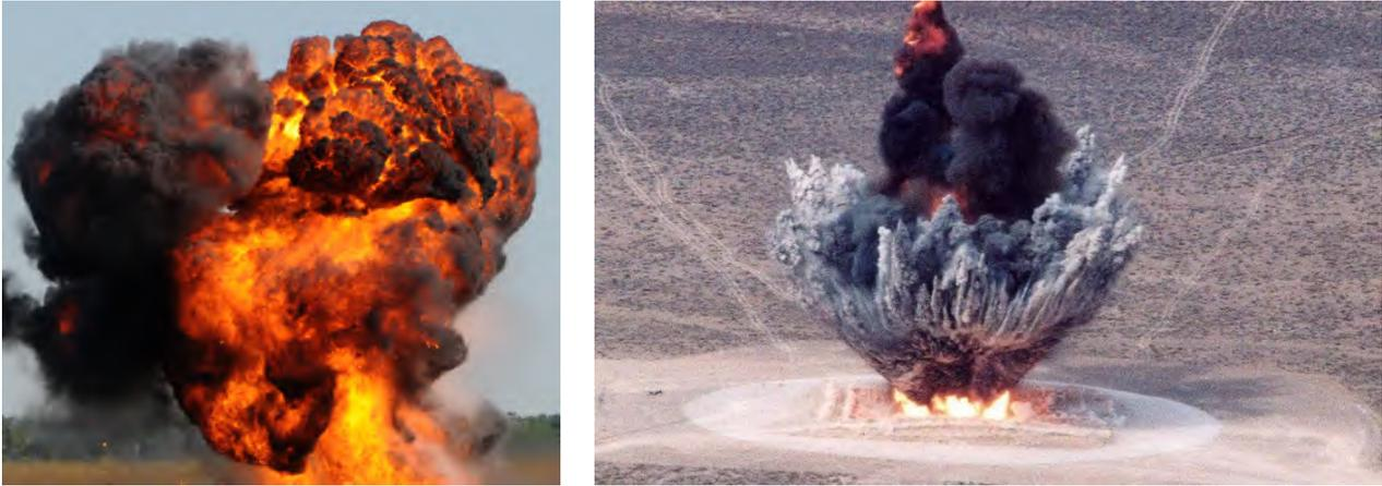
Figure 31: Examples of gasoline “explosion” (deflagration) on the left and true explosion (notice the shock wave on the ground) on the right. Right image is from United States Department of Energy.
