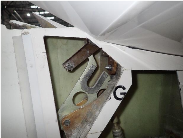
Disconnected elevator control
